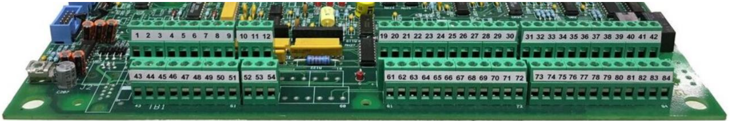
Figure 8: Control Circuit Terminal Locations
