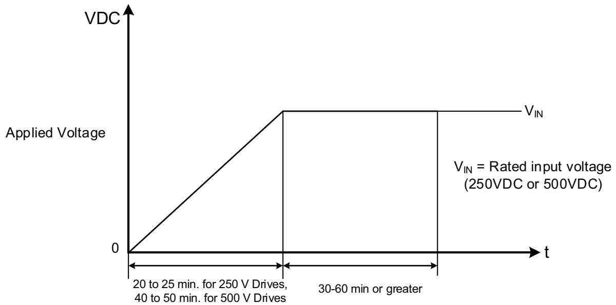
Figure 2-5: DC Bus Capacitor Reforming Timing Diagram
