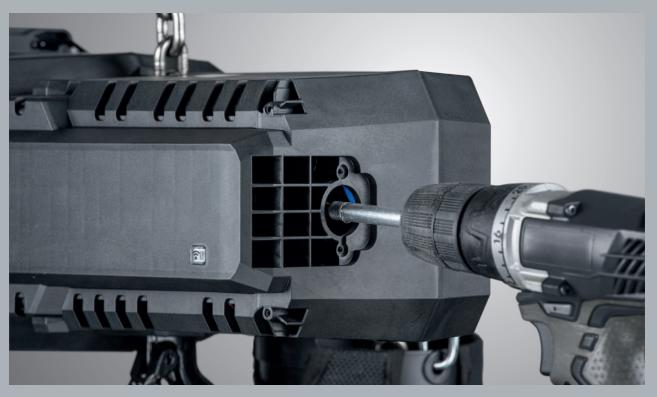
If the battery runs out during hoist operation, the load can be manually lowered. Simply open the end compartment and use a screwdriver or power drill to lower the load.
